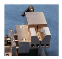
The Brillant 220 Bolt / Fastener vice system is designed to accommodate a wide selection of bolts and fasteners allowing accurate longitudinal sectioning with ease It fits directly on to the Brillant 220 T slot bed or can be combined with the Easy Clamp Base system using the Adapter Plate
