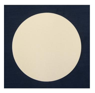
Nylap is a medium hard woven synthetic cloth primarily designed for tertiary grinding of a wide range of materials particularly when rubbing can be a issue. It can be employed with oil, water and alcohol based abrasives to produce flat relief free specimens.
