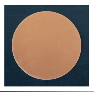
Alphacloth is a synthetic medium napped final polishing cloth with the fibres are bonded to a woven cotton backing. For use with all final polishing abrasives including diamond, alumina or silica abrasives usually in the 1 micron or below size range.
