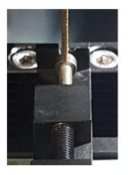
Clamp the Sample in the Miniature Fastener Vice and clamp the Miniature Fastener Vice in the jaws of your standard abrasive cutter vices.
