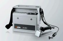
The Qetch 100 M (KRISTALL 650) is a mobile battery supplied electrolytic polisher and etcher. It convinces by its compact and robust construction, ideal for use outside of the lab.
