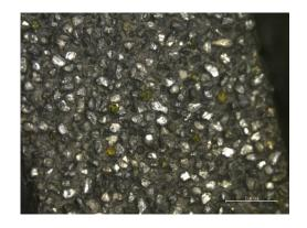
Available in 120 um for rapid stock removal or 30 um for standard grinding - Magnetic backed
