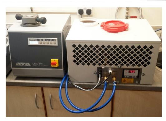
Opal 410 Hot Mounting Press coupled to the dedicated Recirculating / Chiller Unit for the rapid cooling of mounted samples. Ideal for use where no mains water supply is available or a more environmentally friendly cooling water solution is preferred. Product code ATZ 0730007
