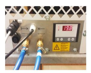
The self contained chiller system & direct plumbing to the mounting press makes connection simple. The operation of the unit is automatically controlled by the mounting press and cooling times are now reduced to typically a couple of minutes. Capacity of the unit is 6 litres.
