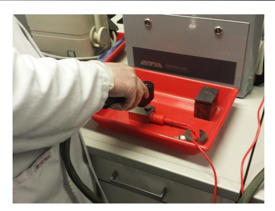
The KRISTALL 650 is a mobile battery powered electrolytic polisher and etcher ideal for both bench top & 'on site' applications. A self contained unit powered by a Lithium battery which allows for typically 150 polishing cycles. Simple to operate with a clear LED display.
