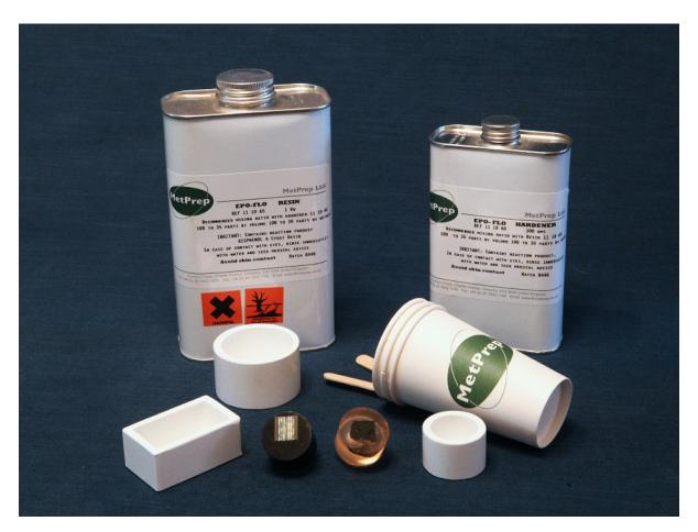
MetPrep's New Ultra-Low Viscosity Epoxy Cold Mounting compound is a two part mixture comprising a resin and hardener system
