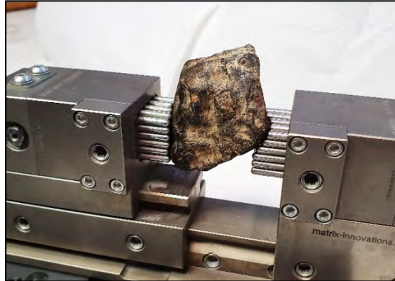
The X- Clamp – Secure clamping of irregular samples without the use of excessive force
