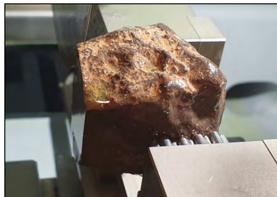
The X- Clamp – Secure clamping of irregular samples without the use of excessive force
