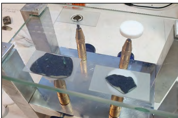
Fig 11 - Ready for mounting, adhering to the glass slides, jiggig & UV cure
