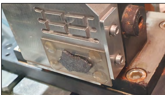
Fig 9 - Surface preparation using a Cup grinding Wheel on the Brillant 220
