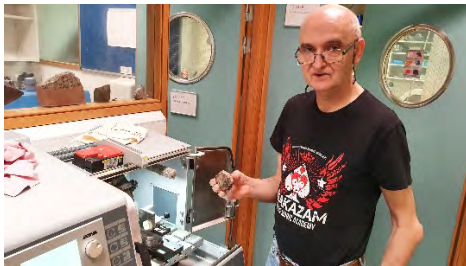
Tony preparing to section the large sample on the Brillant 220
