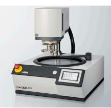
The Qpol 300 A1-ECO is a single-wheel grinding and polishing machine for the metallographic laboratory, suitable for working wheels  $\emptyset$  250/300 mm. The machine is conveniently operated by a 4.3 "touch screen.
