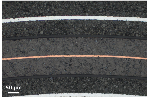
Lithium ion battery. Brightfield, EC Epiplan 20×/0.4
