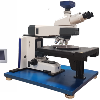
Custom build – 8” wafer microscope with automated stage and focus
